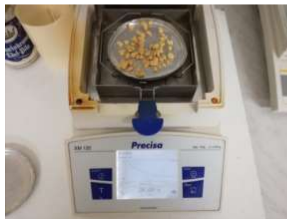
Fig.10. Determination of the moisture content of the biscuit dough (orig.)
