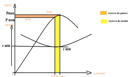
Fig. 4. External feature of the thermal engine
