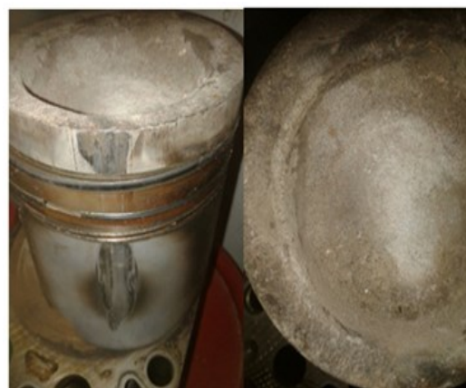
Fig. 3. Degradation of the engine due to the high content of hydrogen sulfide in biodigester
