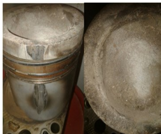
Fig. 3. Degradation of the engine due to the high content of hydrogen sulfide in biodigester (Source: Viquez Saborio C, 2017, [15].)
