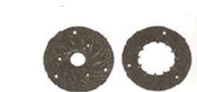
Fig. 2. Burr mill reducing mechanism Source: [6].
