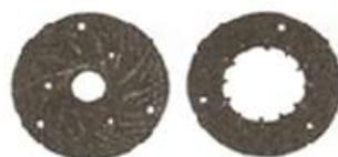
Fig. 2. Burr mill reducing mechanism Source: [6].
