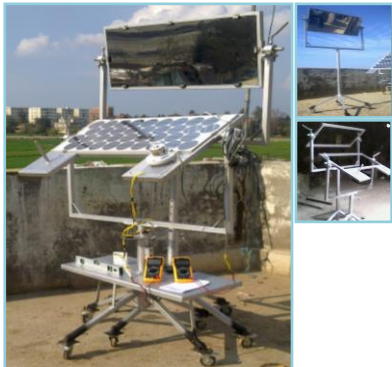
Fig. 1: Augmented device to reflect solar radiation on the PV modules.
