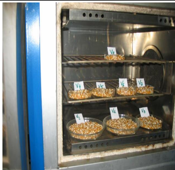
Photo 3. Maize beans subjected to determinations at a 11.9% H
