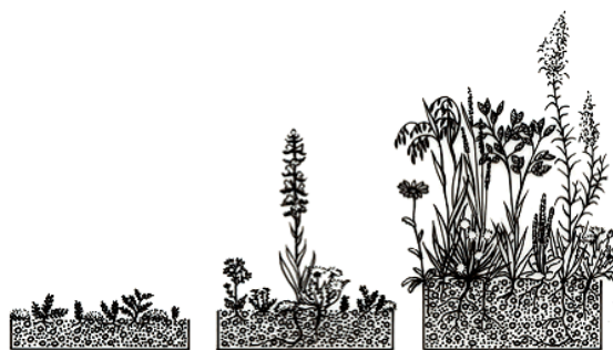
Fig. 1. Different substrate depths (6, 12, and 20 cm) used to create various vegetation forms as a basis for the colonization of diverse fauna on the roof [1].
