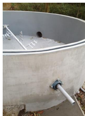
Photo 10. Stirring system using bar horizontally. (Taken from Carlos Saborio's investigation).
