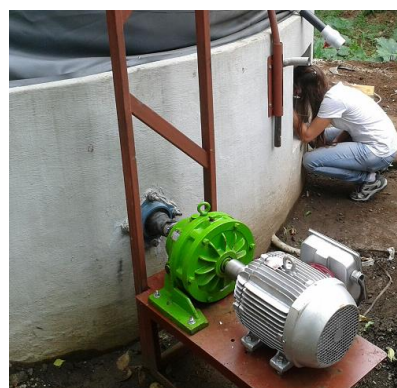
Photo 5. Geared motor for mesophilic digester agitation in the form of horizontal bar. (Taken from Carlos Saborio's investigation).
