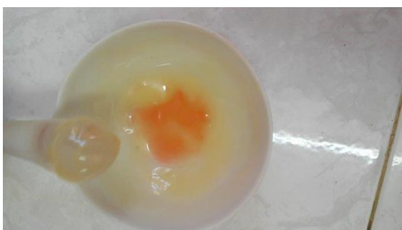
Photo 2. HMF identification method Fiehe (orig.)
