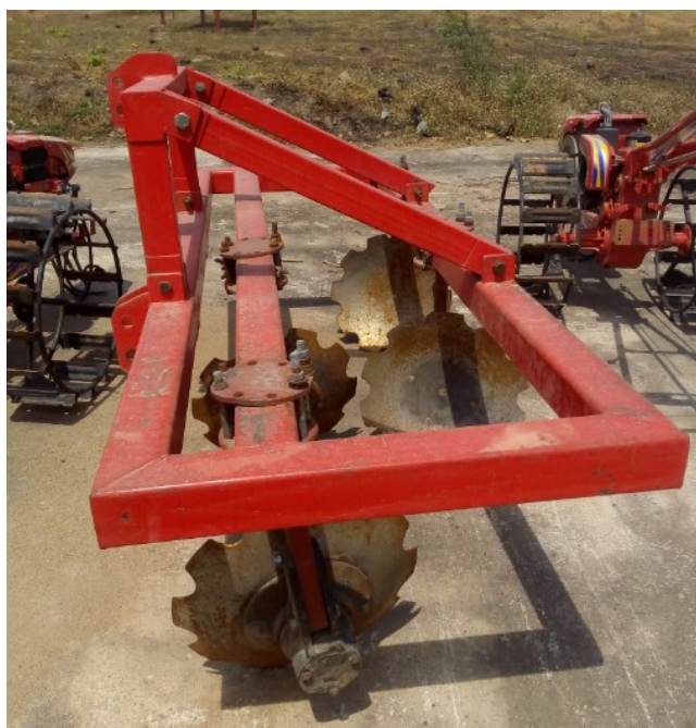
Photo 4. New improperly fitted supposed Disc Ridger
