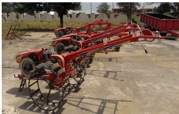
Photo 5. New Non-funtional Power tileings resulting from supply of incomplete components and left under direct sunshine and rainfall
