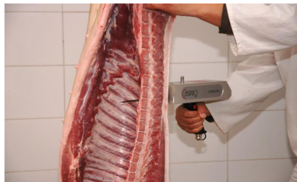
Fig. 4. Optigrade Pro (OGP) optical classification method, 2016
