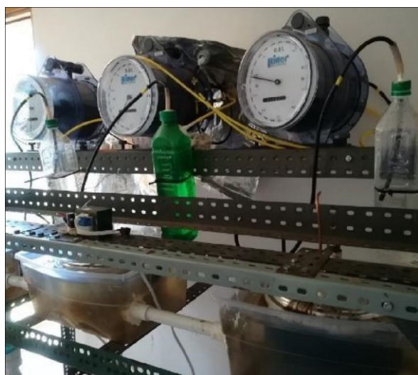
Fig. 4. Assembly of fermentation test with 6 liters biodigesters.
