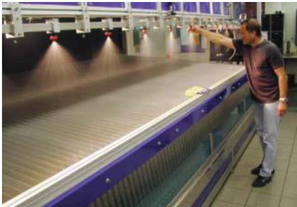
Fig. 1. Bank for determining the working indices of spraying machines Source: [9]
