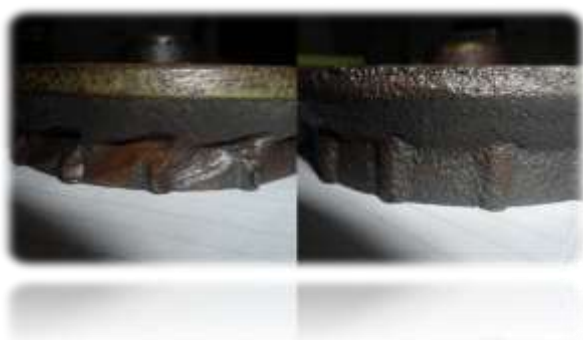
Fig.4. Corner wheel before and after wearing Source: Author's own illustration.
