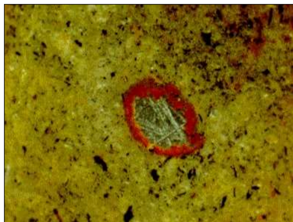
Fig. 2 Black redoximorphic features in soil matrix and red ferric pseudomorphosis on a bio-pore wall
