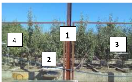
Fig. 4. Phytomonitoring for 72 hours in hair trees. 1- general appearance; 2- PTM -48 A apparatus; 3- measuring room; 4- RTH-48-weather module + measuring chamber. Source: Original photo.
