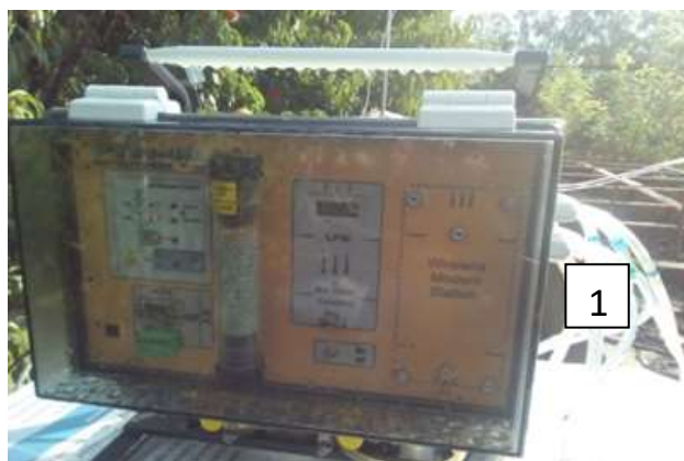
Fig. 2. PTM-48A phytomonitoring device in operation immediately after rain. Source: Original photo.
