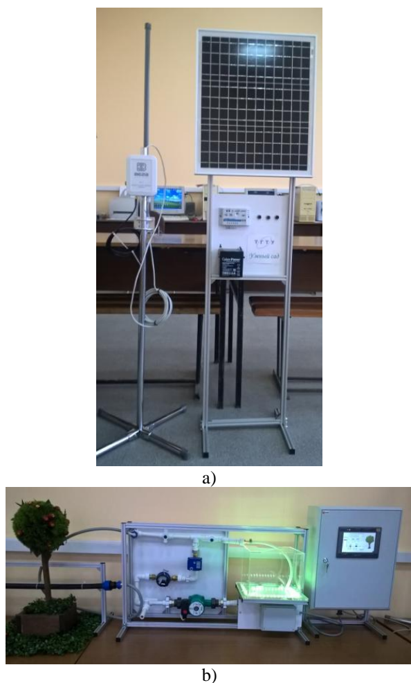
Fig. 4. Basic station BS2 and uninterrupted power supply (a), actuating subsystem of drip irrigation (b) Source: Compiled by authors.
