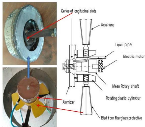
Fig. 1. The diagram of fabricated an electric rotary cage atomizer
