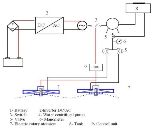
Fig. 2. Two rotary cage atomizers in the completely prototype sprayer with electricity circuit and water line. Source: Authors' own illustration.
