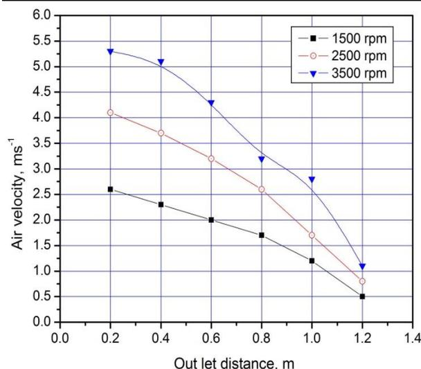
Fig. 5. The produced air velocity from single developed electric rotary cage atomizer at different rotational speed.
