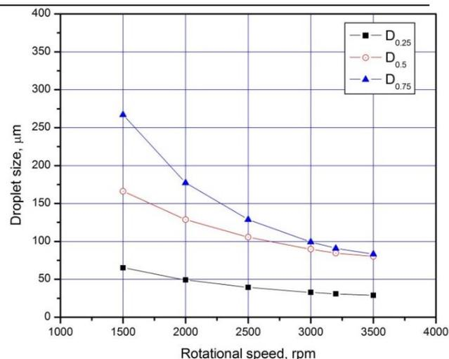
Fig. 6. The droplet size predicted of developed electric rotary cage atomizer at different rotational speed at maximum air velocity  $5.3 \text{ ms}^{-1}$  and maximum flow rate  $1.4 \text{ l min}^{-1}$ .
