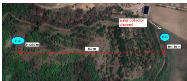
Fig. 10. The ponds positions and dimensional parameters
