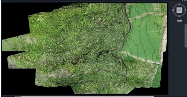
Fig. 8. The resulted orthophotoplan and 3D DTM for the surveyed area
