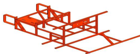
Photo 2. The main frame of the manufactured rice transplanting machine Source: Authors' drawing.
