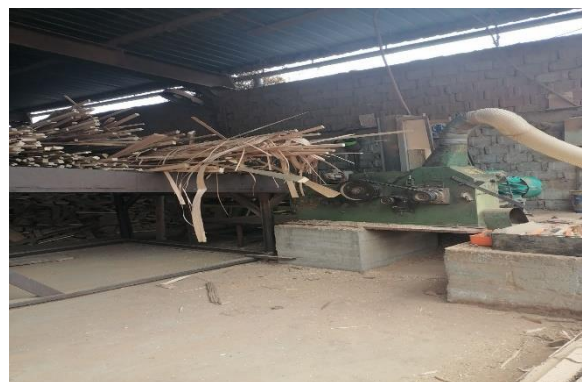
Photo 9. Equipment for shredding large-sized wood waste Source: Original S.C. AmisMob.
