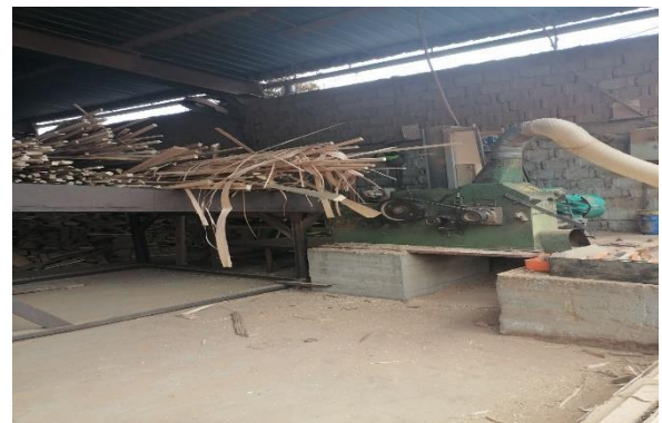
Photo 9. Equipment for shredding large-sized wood waste Source: Original S.C. AmisMob.
