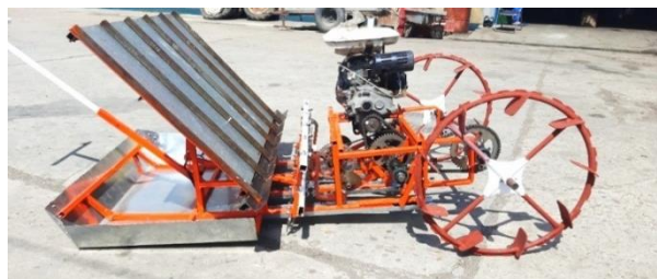
Photo 1. The manufactured rice transplanting machine Source: Authors' own illustration.
