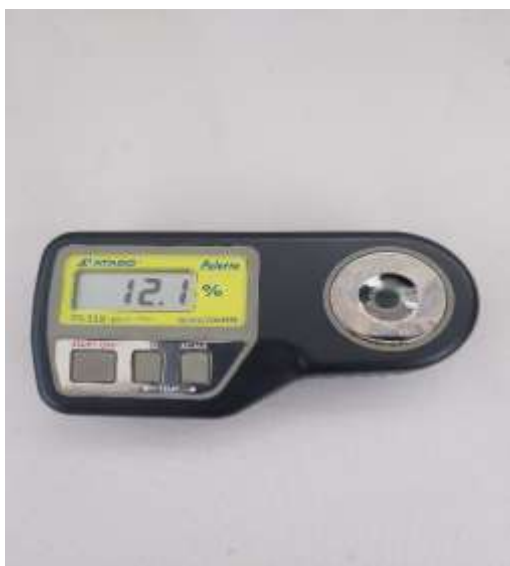
Photo 6. Soluble dry matter determination, using the Atago refractometer Source: Original.
