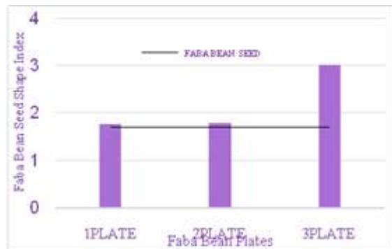
Fig. 15. The relation between the shape index of faba bean seeds and the holes in various metering plates Source: Authors' determination.
