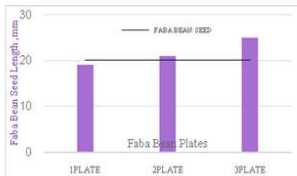
Fig. 7. The relationship between the length of faba bean seeds and the length of holes in various metering plates Source: Authors' determination.
