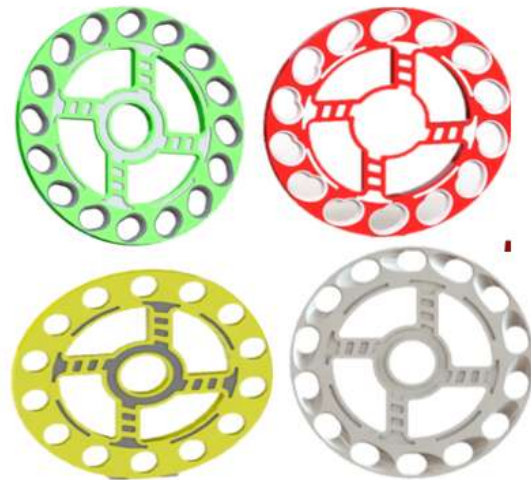
Fig. 2. Faba Bean Metering Plates Source: Authors' determination.
