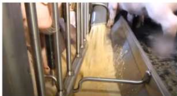
Photo 3. Spotmix II feeding system (Schauer) for the preparation of liquid feed for pig complex No. 3 (Demydivka village)
