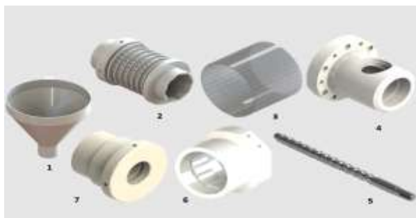
Photo 2. Parts of extruder machine Source: Author's' determination.
