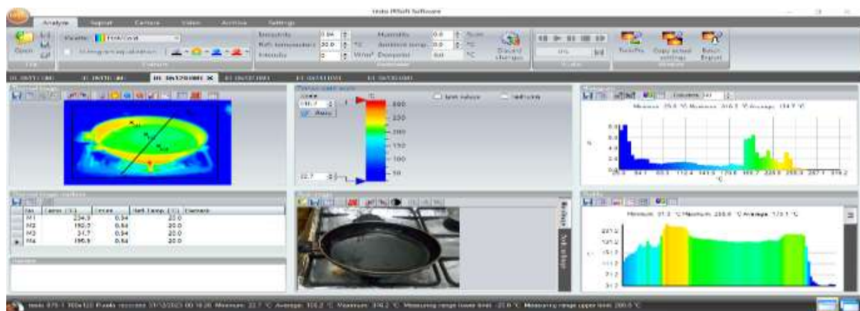
Photo 15. The internal temperature of Tefal Skillet, the temperature of air, oil and potato by IRSoft software
