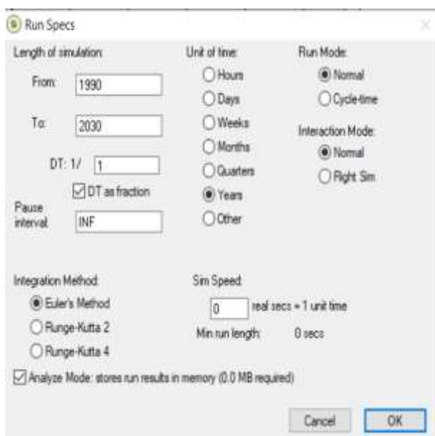
Fig. 16. Fragment of the STELLA program with setting of simulation parameters according to the Euler method Source: authors' own calculations from STELLA program.
