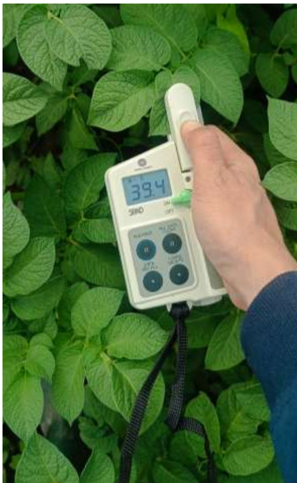
Photo 2. Measuring the chlorophyll content with the SPAD-502PLUS device, on a potato leaf from the experimental field in Rusciori Source: Original by own determination
