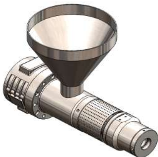
Fig. 1. Fish oil extruder machine Source: Authors' designed.
