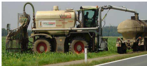
Fig. 3. Vehicles for application of digestate as fertiliser, using dragging hoses (AGRINZ 2008)
