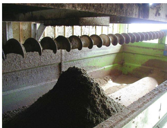
Fig. 4. Fibers collection wagon with distribution screw (ANGELIDAKI, 2004)
