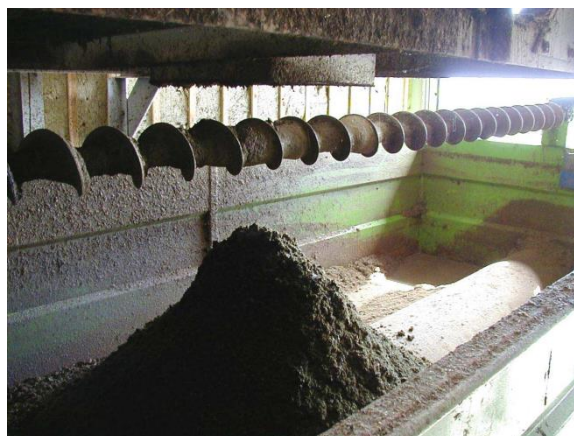
Fig. 4. Fibers collection wagon with distribution screw (ANGELIDAKI, 2004)
