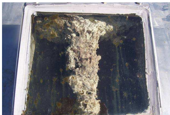
Fig. 3. Elementary sulphur resulted from biological desulphurization inside the digester [9]
